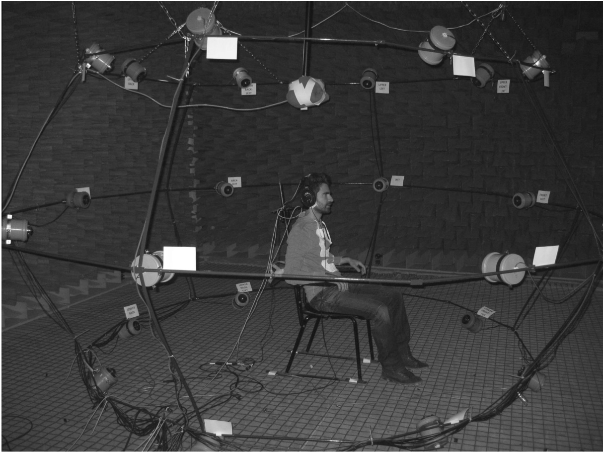
Fig. 5. Anechoic room with loudspeaker setup and subject.
