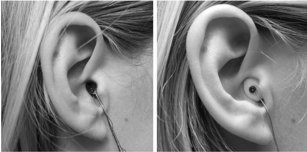
Fig. 2. Miniature microphone placed at the entrance of the ear-canal using an Open-Dome (left) and an ear plug (right).
